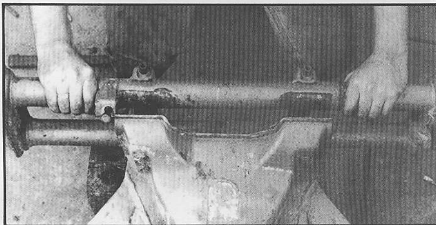
The torsion bars and complete front suspension can now be removed.
