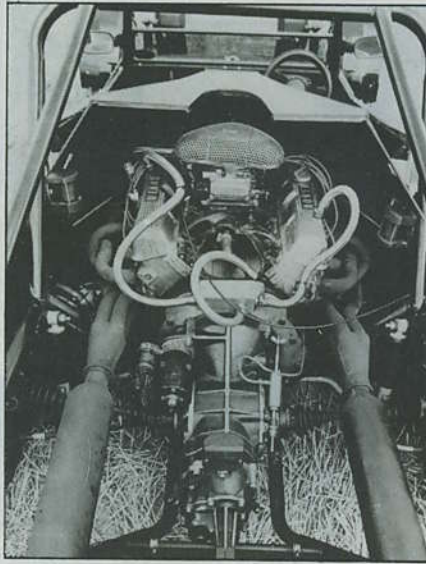
The heart of the matter ( above ); the Rover V8 with Holley four-barrel produces 230bhp. The interior ( below ) is not the last word in comfort
