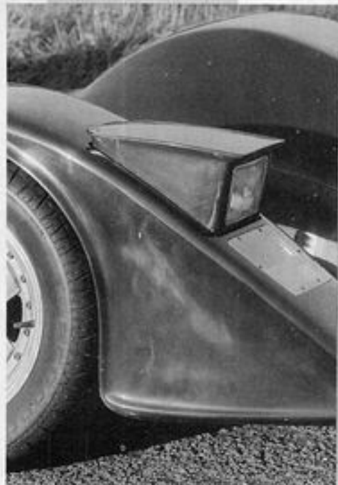
Above: Pop-up headlights are operated by a simple choke-type cable rather than a motorised set-up, to save on weight and cost
